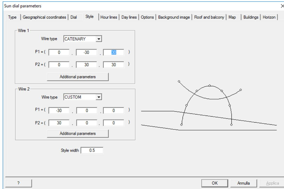
Select the desired wire type from the combo box and insert the end points in the P1 and P2 fields. For catenaries and custom wires the button «Additional parameters» allows to introduce additional data.
