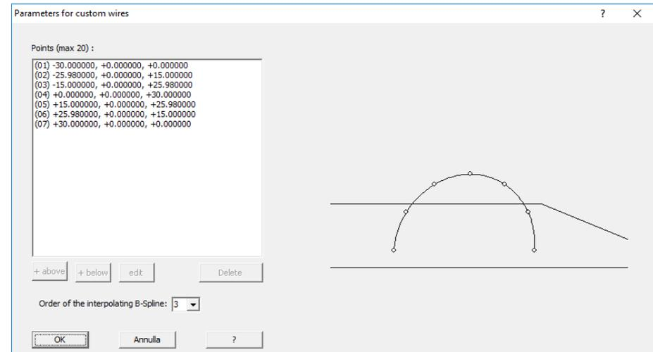
Points coordinates are defined in a reference system (common to every section of the program) where **x** and **y** axes lay on the dial plane, x rightward and y downward, and the **z** axis is perpendicular and coming out of the dial plane. Origin position is arbitrary.
