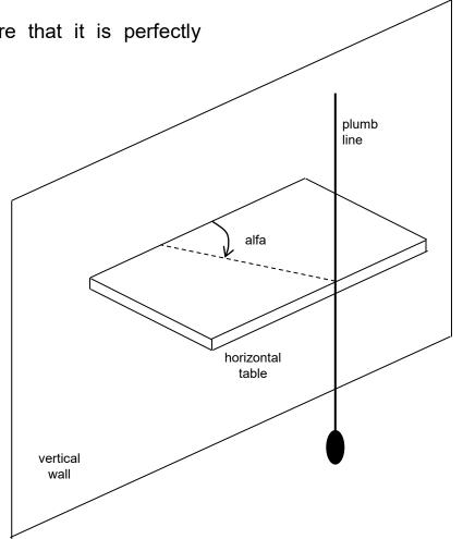
To perform the measurement an instrument similar to the the one shown here can be prepared.
